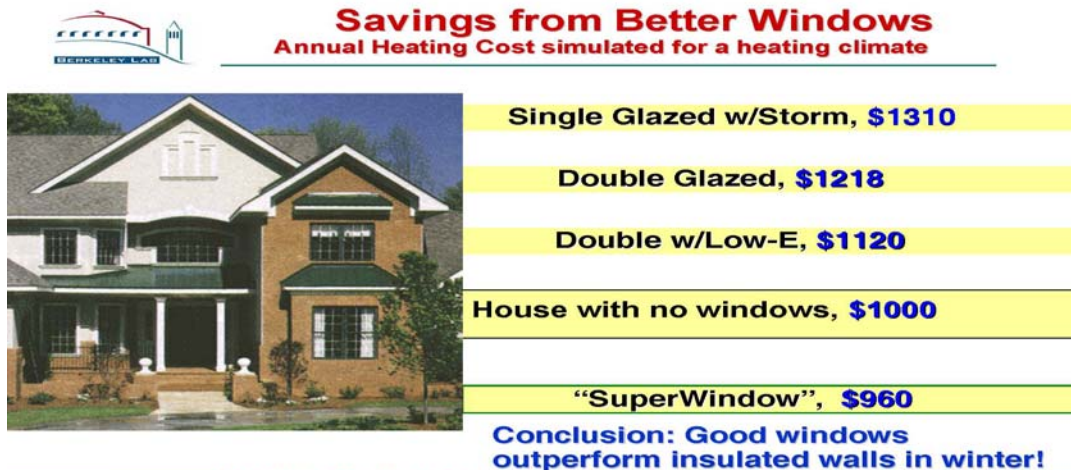
Figure 3 Simulated winter seasonal energy use of a house in Boston as windows are improved; note that the house with "super windows" with U < 0.15 has a lower winter heating bill than the same house without any windows so the windows are now net energy suppliers. Reprinted with permission from the Department of Energy's Lawrence Berkley National Laboratory.
